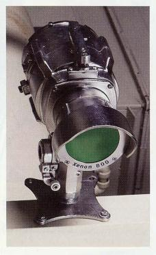
MSA's SafEye Xenon 800 Gas Detection System detects a wide range of hydrocarbons over an open path of up to 120 meters. The system is resistant to false alarms and poisoning, and it has operational records in an extremely wide range of climates. The combination of triple optics and dual-spectrum sensor allows the system to maintain operational integrity in up to 90% signal obscuration. For more inf<sup>o</sup>rmation contact: MSA, (800) 672-2222, www.msanorthamerica.com.
