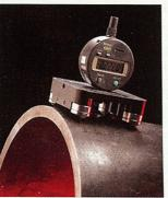
Exacto Machine of Indianapolis, IN, announces that its new Rolling Pit Gauge is the ideal tool for assessing corrosion pits that occur on the circumference of pipe. The pit-depth gauge can be moved in a 360-degree motion to find the deepest part of any anomaly.
